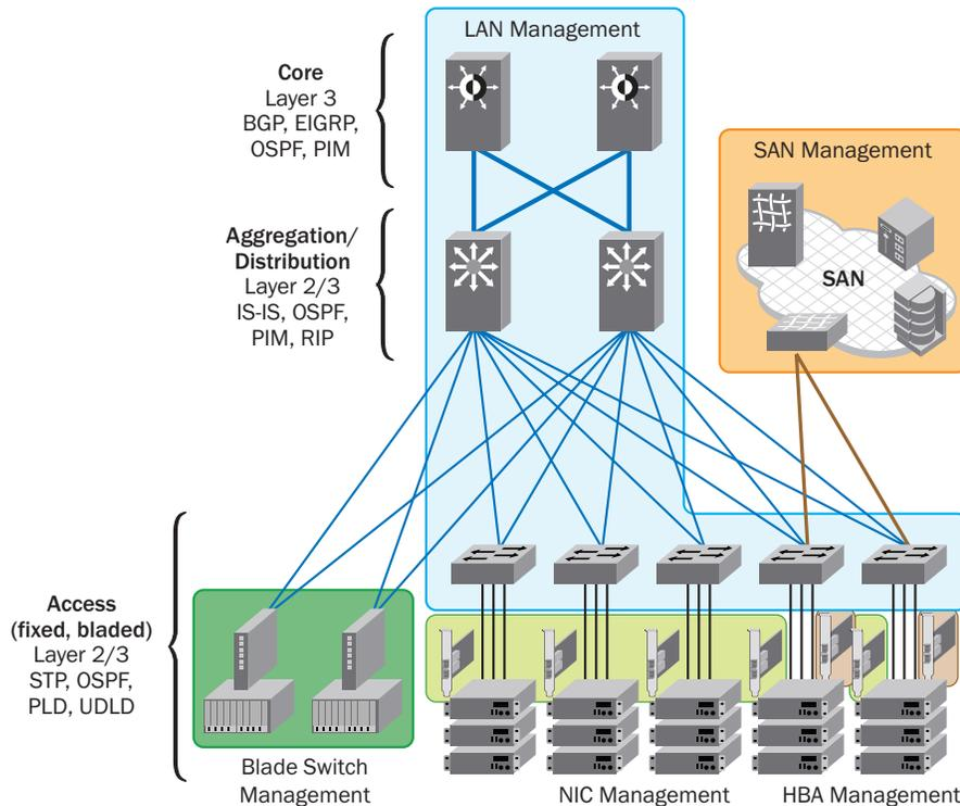
**Figure 4.** Multi-tier network architectures and many Layer 2 and 3 protocols increase complexity and drive up management costs.
