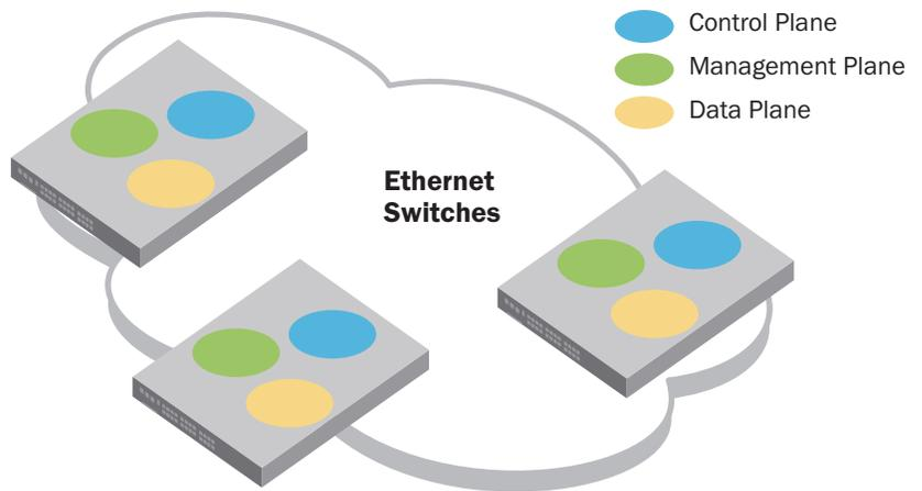
Ethernet fabrics can be thought of as extending the control and management planes beyond the physical switch into the fabric. As shown in Figure 3, they now operate at a fabric level rather than at a switch level.
