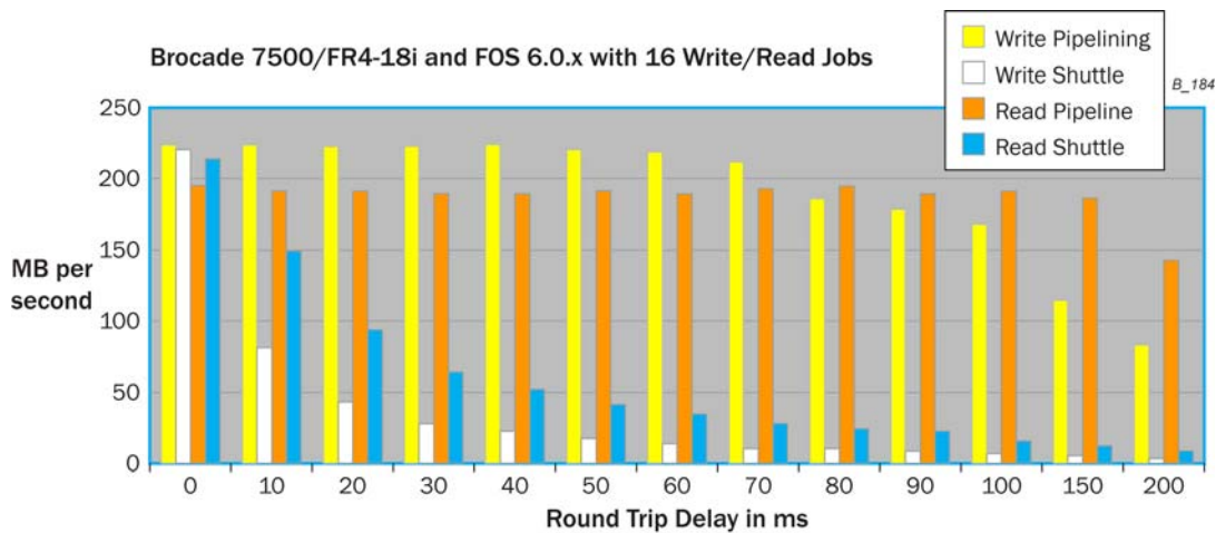
Figure 5. FICON tape read/write pipeline performance for 4 VTCs and 16 read/write jobs
