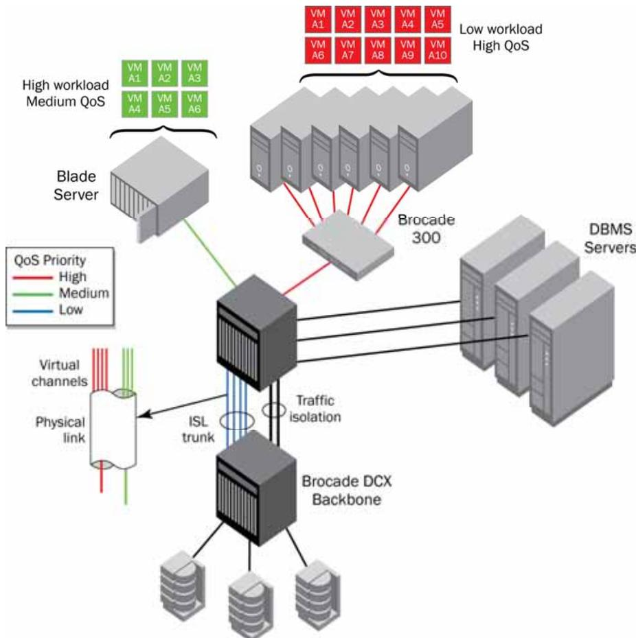
Figure 4. Adaptive Networking services simplify fabric management
