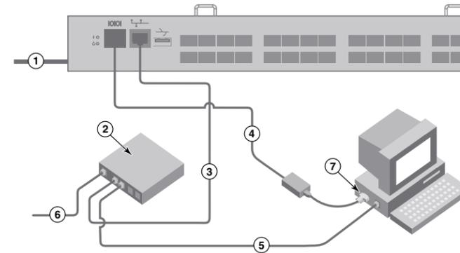
1. Connect the power cord to the switch and to a power source (1). The power and status LEDs display amber then green. This can take from one to three minutes.
